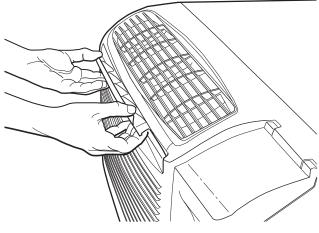
FIGURE 17 — INDOOR-AIR INLET FILTER REMOVAL
